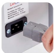
IEC power cable into the mains.
